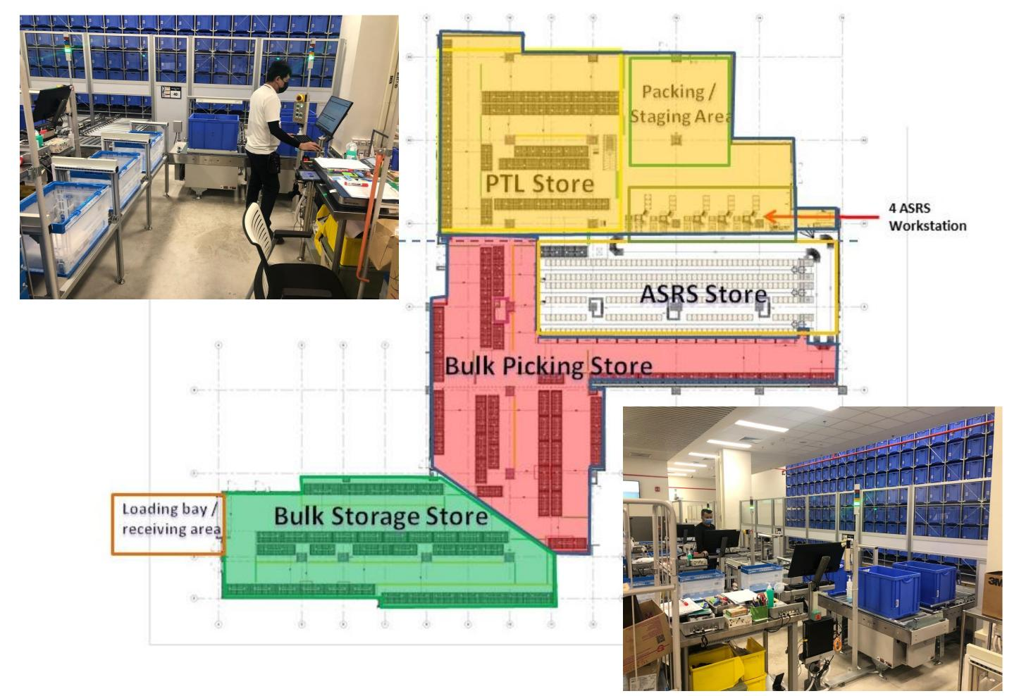
The ASRS has been designed for future expansion in terms of a 5<sup>th</sup> workstation and additional capacity of automated storage transporter vehicles. The integrated system allows the dynamic movement of line items between ASRS and PTL and between PTL and Bulk Picking store.
